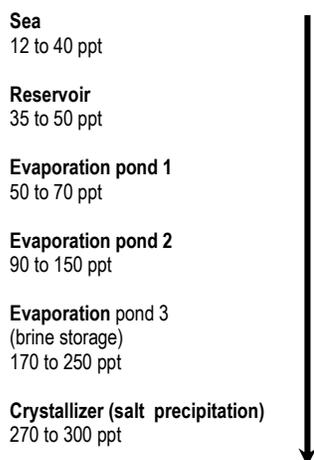
**Fig. 5: Scheme of a salt street in Vinh Chau, Mekong Delta, Vietnam, with direction of seawater flow into consecutive ponds prior to salt precipitation (not to scale).**
